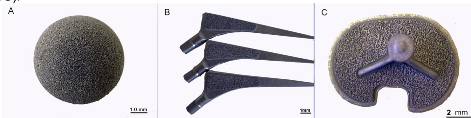
Fig.1 Prototypes of porous titanium (alloy) orthopaedic implants made by sponge replication: (A) Acetabular cup for total hip joint replacement; (B) Porous Ti6Al4V as coating on hip stem, (C) Porous titanium as coating on tibia tray.
